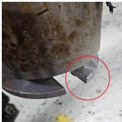
Incident 1: Scarring observed on the anti-two block
