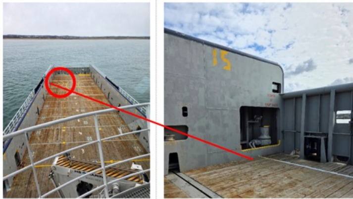
Bridge view - Capstan winch located inside crash rail
