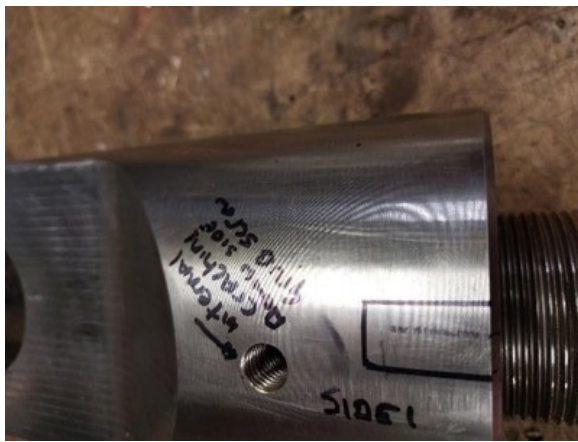
Side 1 Defect grub screw hole
