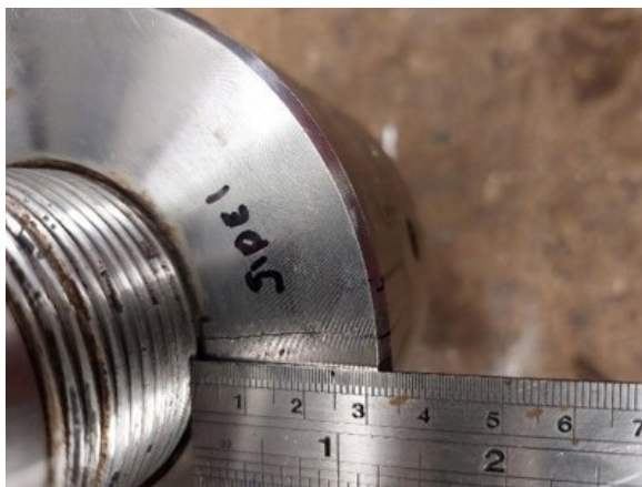
Side 1 Thro' wall defect
