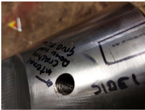
Side 1 Defect grub screw hole
