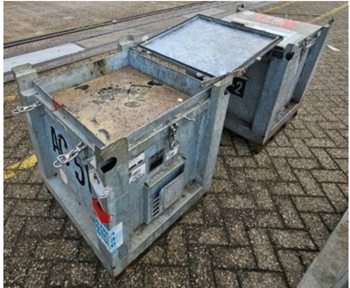
Faulty batteries safely removed from the vessel and submerged in water containers on the quay
