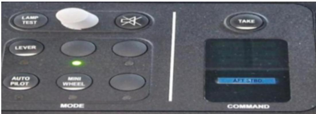
Upon returning to the DP station, the vessel was found in manual LEVER mode instead of DP Mode. Amber alerts were issued to the ROV and crane; the ROV began returning to the TMS, and the crane lifted off the seabed.
