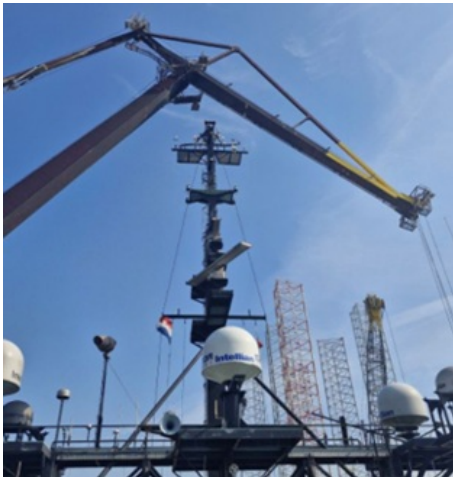
Boom adjacent to mast after the incident
