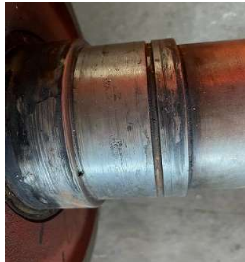
Rotor of Shaft generator/ failed bearing part caused overheating and smoke
