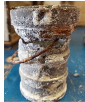
Damage to failed fire hose coupling
