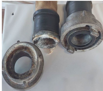
Damage to failed fire hose coupling
