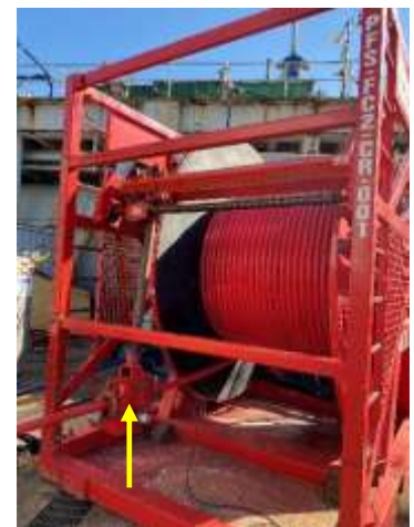
Incident 1: The spot where the contractor's right thumb was pinched between the ball valve and the horse head.
