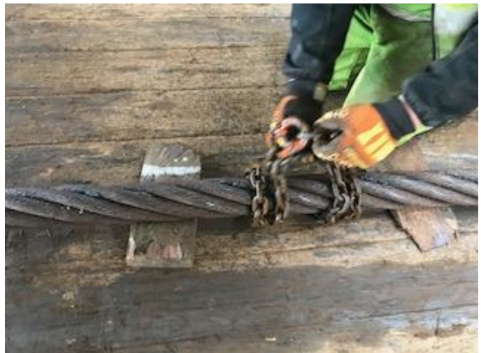
Disconnection of the chain (post-incident solution)
